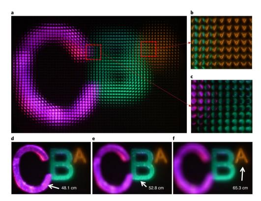
**Fig. 2** | Characteristics of the radiance captured by the focused metalens array light-field-imaging system. **a**, The raw light-field image with the achromatic metalens array. Three letters made from plastic are arranged neatly in the intermediate image space under halogen lamp irradiation (purple C, green B and yellow A). **b,c**, Zoomed-in images of **a**. **d-f**, Rendered images with focusing depths of 48.1cm (**d**), 52.8 cm (**e**) and 65.3 cm (**f**).
