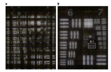
**Fig. 4 | Quantification of the imaging resolution of the light-field system with an achromatic metalens array. a**, Raw light-field image of the 1951 United States Air Force resolution test chart. **b**, The rendered image of **a**. The white dashed line marks the smallest resolvable target of this system (group 8, element 1).
