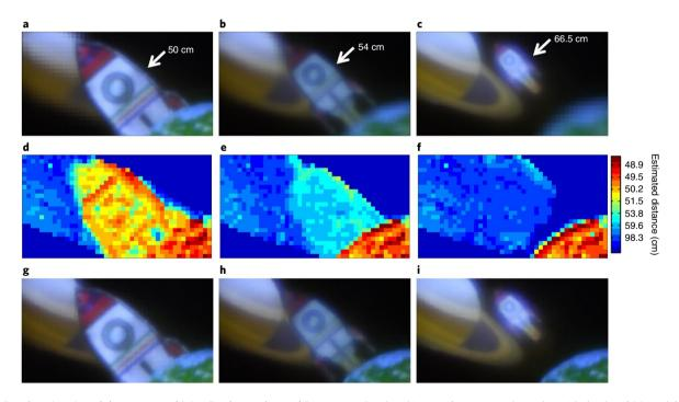
Fig. 3 | Depth estimation of the scene combining Earth, a rocket and Saturn. a-c, Rendered images focusing on the rocket with depths of 50 cm (a), 54 cm (b) and 66.5 cm (c). d-f, The estimated depth maps corresponding to images a-c. g-i, Rendered all-in-focus images with the rocket at different positions between Earth and Saturn.
